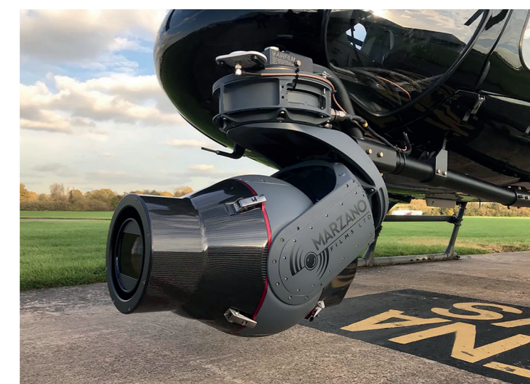
The Mini Eclipse is the latest state-of-the-art gyro-stabilised system for helicopters, aeroplanes, boats and tracking vehicles. It is the only compact sub 70kg platform that can take the super-large lenses such as the Angénieux Optimo 28:340 and Panavision Primo 11:1 zooms. It has GPS tracking capability and the only true fixed horizon due to the unique integration between its inertial measurement unit and GPS receiver
